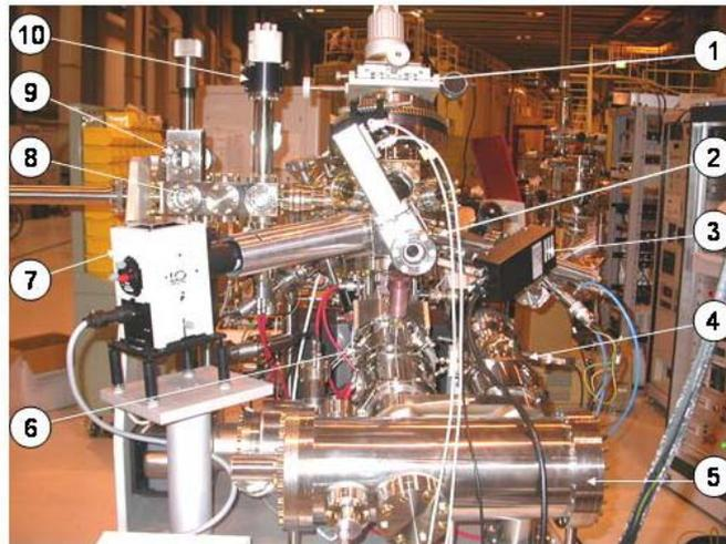
Fig. 2. Front view of the SPELEEM instrument. 1, manipulator, 2, photon incident port, 3, quadrupole mass spectrometer, 4, projector column, 5, energy analyzer, 6, image column, 7, Hg lamp, 8, preparation chamber, 9, air lock, 10, sputter ion gun.
