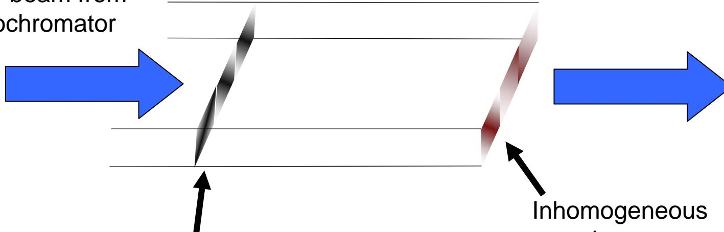
X-ray flux is not homogeneous and the density pattern moves and changes along with the monochromator angle scan
